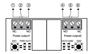
Use to open door: When user press button to open door, its make button two lines connect 1-2 seconds, then disconnect. It can connect two lines to COM and NO terminal, calling the device, it will connect COM and NO terminal for 3 seconds; then its like you press the button and open the door.
